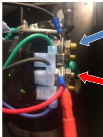
Attach battery negative (ground) to contactor here (6 gage min)
