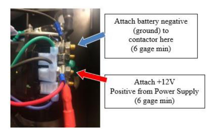
**Pump Ground** Attach a # 6 gauge (minimum) wire between the negative -12 volt terminal on the battery and the negitive terminal on the contactor as shown in Fig.2. These unts will not ground thru the mounting. The decribed ground/negitive battery to contactor connection must be made.
