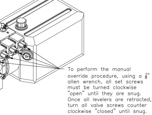
Manual override screw,\_ 1/4" allen head, is under this sticker. Using a 2000 rpm minimum drill, retract jacks by turning counter clockwise. To extend, turn screw clockwise.
