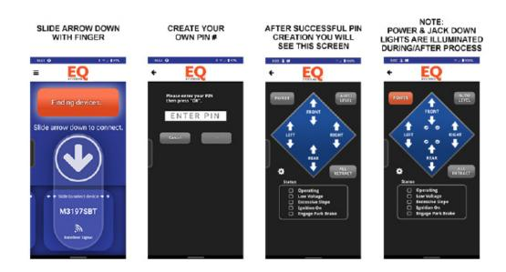
Note: The All Retract button will only retract the rear (and center jacks on a 6 point) on a trailer system. Use the manual arrow for the front jacks once the trailer is connected to the tow vehicle.
