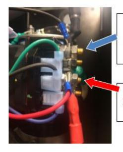
Attach battery negative (ground) to contactor here (6 gage min)
