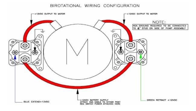
Wiring for Pump # 3040, 3041, 3200, 3201 and 3201KS
