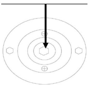
Your hydraulic motor is equipped with a manual override output shaft. The drill must be capable of producing a minimum of 2000 rpm for the pump to develop appropriate pressure output.
