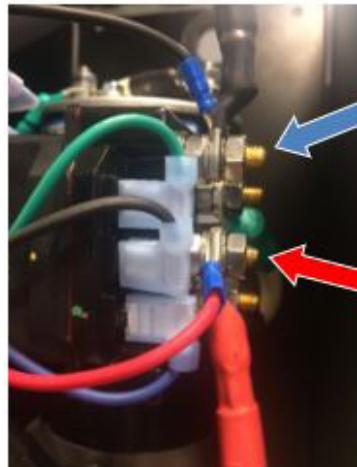
Attach battery negative (ground) to contactor here (6 gage min)
