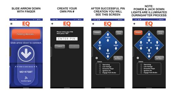
Note: The All Retract button will only retract the rear (and center jacks on a 6 point) on a trailer system.
