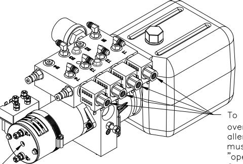
Manual override screw, 6mm allen head, is under this sticker. Using a 2000 rpm minimum drill, retract jacks by turning counter clockwise. To extend, turn screw clockwise. To perform the manual override procedure, using a  $\frac{1}{8}$ " allen wrench, all set screws must be turned clockwise "open" until they are snug. Once all levelers are retracted, turn all valve screws counter clockwise "closed" until snug.
