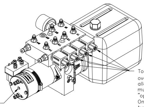
Manual override screw,\_\_6mm allen head, is under this sticker. Using a 2000 rpm minimum drill, retract jacks by turning counter clockwise. To extend, turn screw clockwise.
