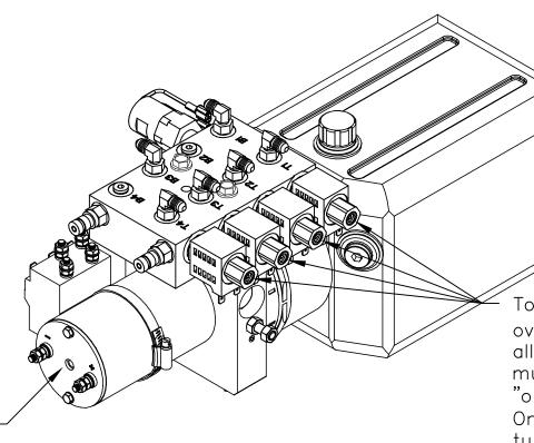
Manual override screw,\_ 1/4" allen head, is under this sticker. Using a 2000 rpm minimum drill, retract jacks by turning counter clockwise. To extend, turn screw clockwise. To perform the manual override procedure, using a ½" allen wrench, all set screws must be turned clockwise "open" until they are snug. Once all levelers are retracted, turn all valve screws counter clockwise "closed" until snug.
