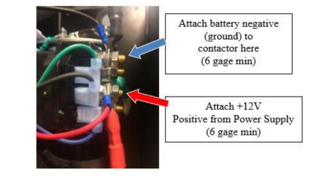
**Pump Ground** Attach a # 6 gauge (minimum) wire between the negative -12 volt terminal on the battery and the negitive terminal on the contactor as shown in Fig.2. These unts will not ground thru the mounting. The decribed ground/negitive battery to contactor connection must be made.
